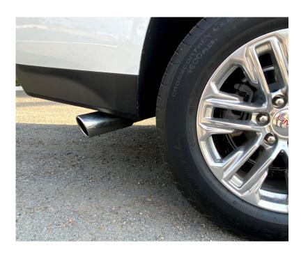
GIBSON EXHAUST systems are designed on a factory stock vehicle. Any aftermarket products installed could increase the sound levels of this Exhaust. Make sure there is a 1" clearance from ALL rubber brake lines, shock boots, fuel lines, tires, etc to prevent heat related damage or fire.
